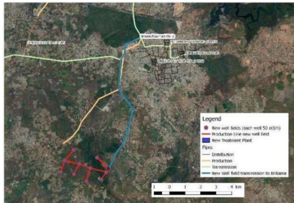
Figure 36: Transfer line layout between the new well-field and Brikama WTP (in blue on the map)
